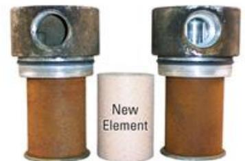
The inlet port shows evidence of poor quality air, whereas the outlet port appears as clean as if it were just machined.
